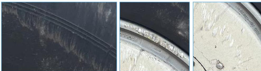
Fig. 15 Abrasion to tyre sidewall, wheel rim, and wheel cover
